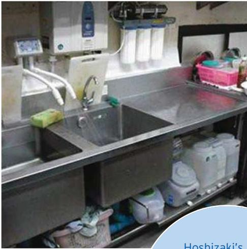
Hoshizaki's ROX produces both sanitizing rinse and alkaline cleaning solution through a membrane-based water electrolysis process.
